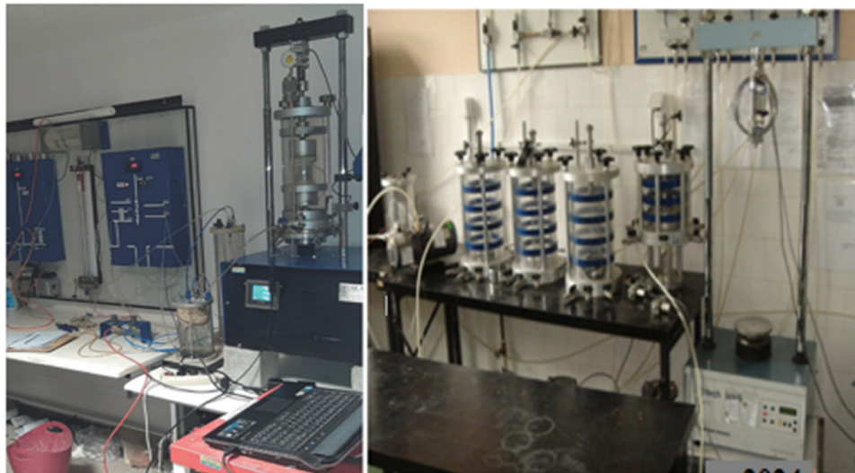
Figure 5. Triaxial tensile test device.
