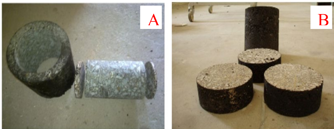
Figure 2: A) Core and trimmed specimen along with waste rings for SPT; B) core specimens for IDT.
