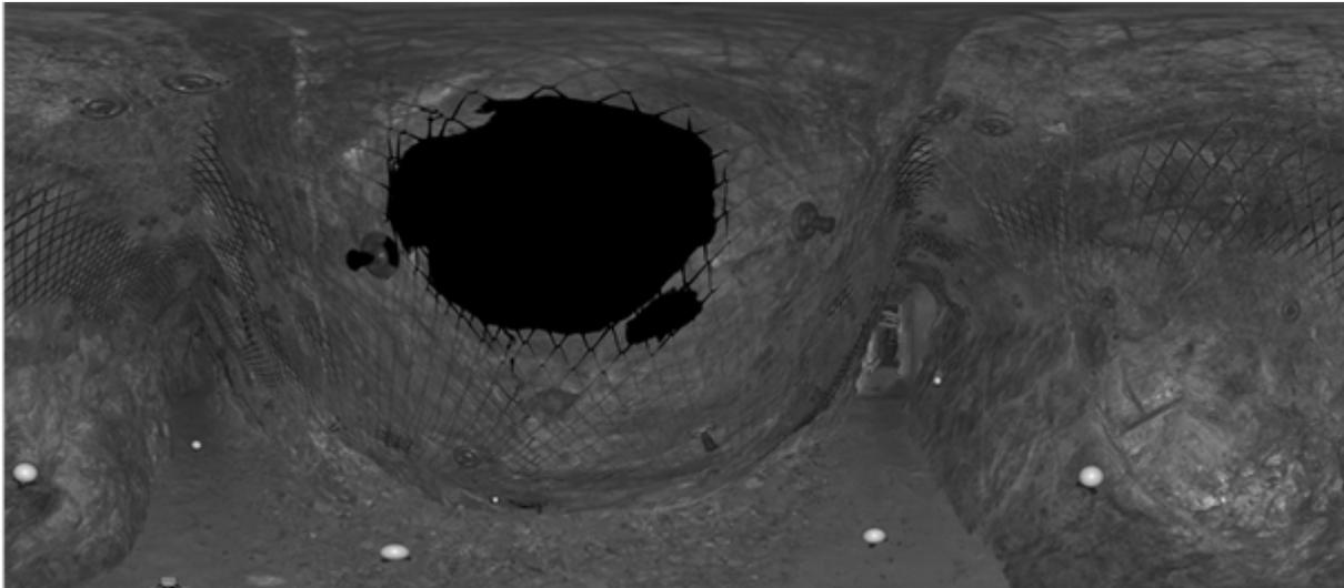
**Figure 4:** The intensity of the laser beam reflection in the adit (the black spot is a fragment of the sidewall closer than 60 cm from the scanner).
