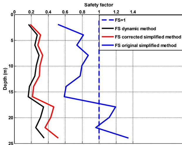
**Figure 12:** Safety factor according to the depth computed by the original and corrected versions of the simplified method (Coastal road Skikda site).
