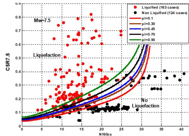
Figure 2: Bayesian mapping function along the case history database using the original version of the simplified procedure. CSR = cyclic stress ratio.
