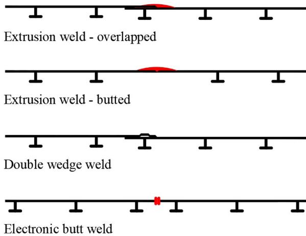
Figure 5: HDPE weld types.
