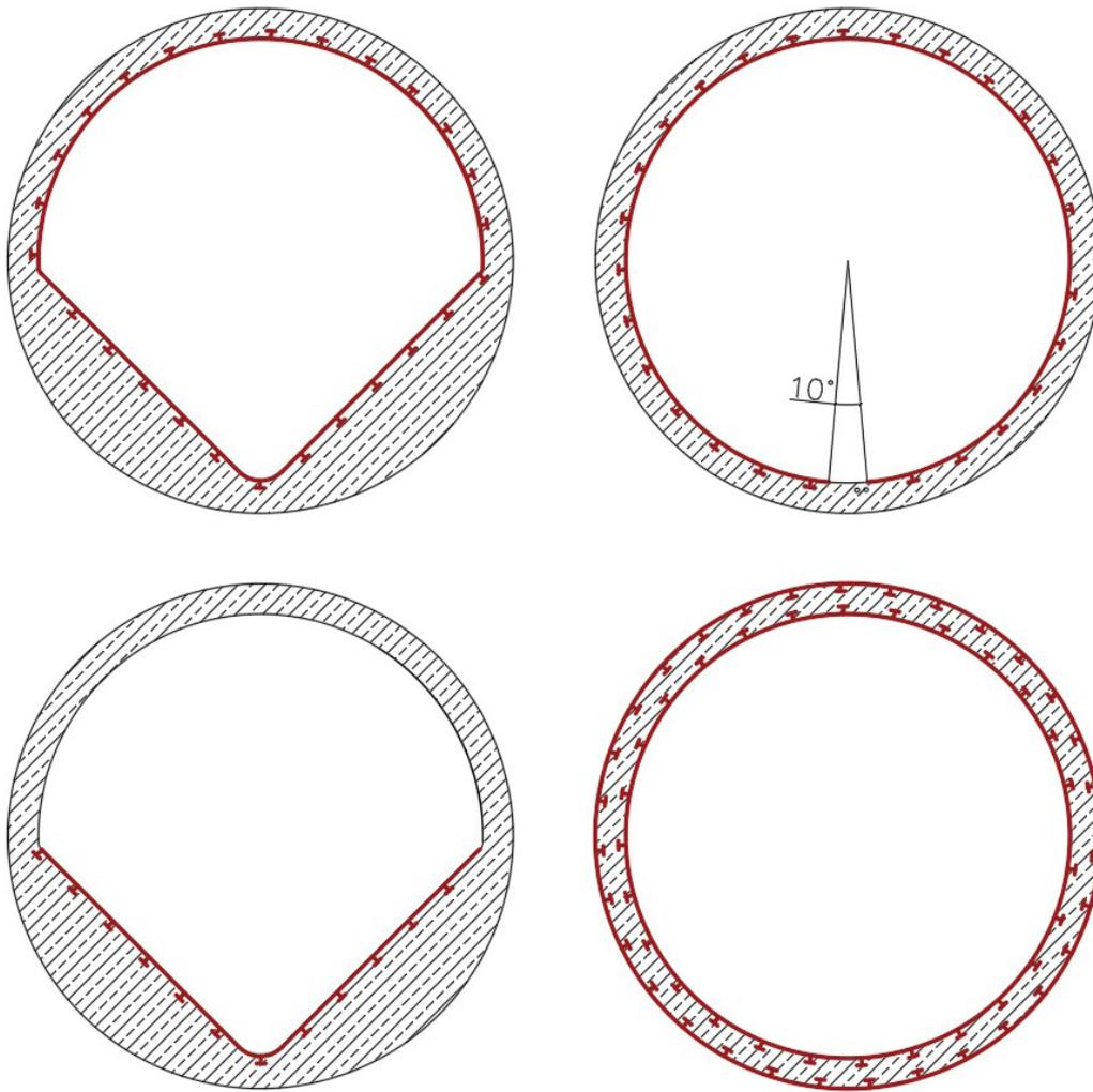
Figure 6: Different installation details of HDPE liners.
