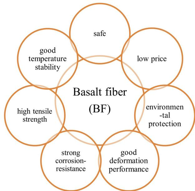
Figure 3: Features of basalt fibre.
