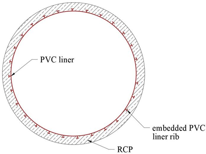
Figure 7: Reinforced concrete pipe with PVC liner
