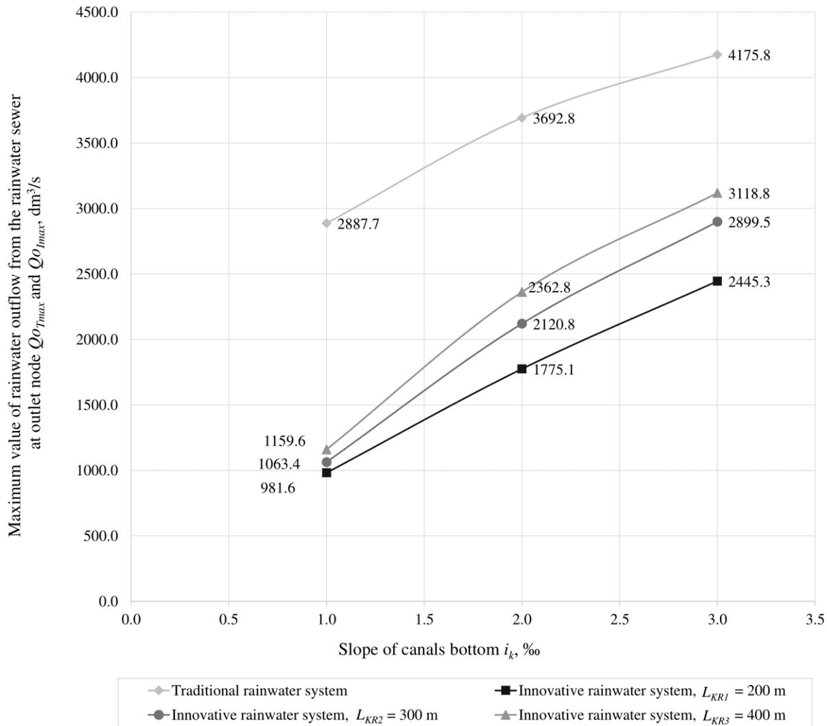
**Figure 7:** Maximum rainwater outflow at the outlet from the drainage catchment for traditional storm water system  $Q_{o_{Tmax}}$  and innovative storm water system  $Q_{o_{I_{max}}}$ , catchment area  $F = 80$  ha (developed on the basis of [1]).
