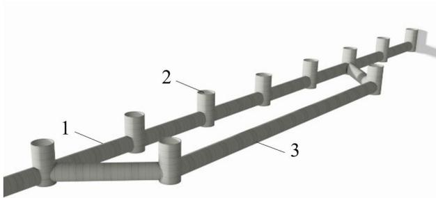
**Figure 2:** An example of an additional transit canal (1 - sewer canal, 2 - sewer manhole, 3 - additional transit canal) [28].
