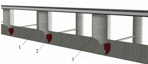
**Figure 3:** An example of a rainwater system equipped with a retention sewage canals (1 - canal, 2 - piling partitions, 3 - manhole) [28].
