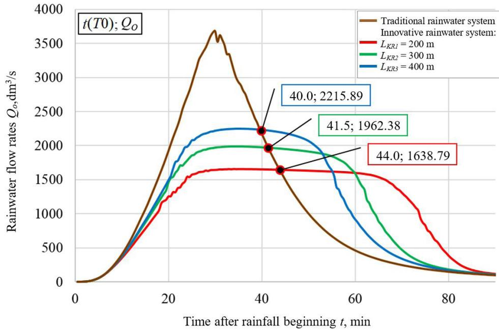
Figure 8: Hydrograms of rainwater outflow from the traditional and innovative sewer system at rainfall duration  $t_d = 25$  minutes, drainage catchment area  $F = 80$  ha, canal bottom slope  $i_k = 2$  ‰ and surface runoff coefficient  $\Psi = 0,5$  [1].
