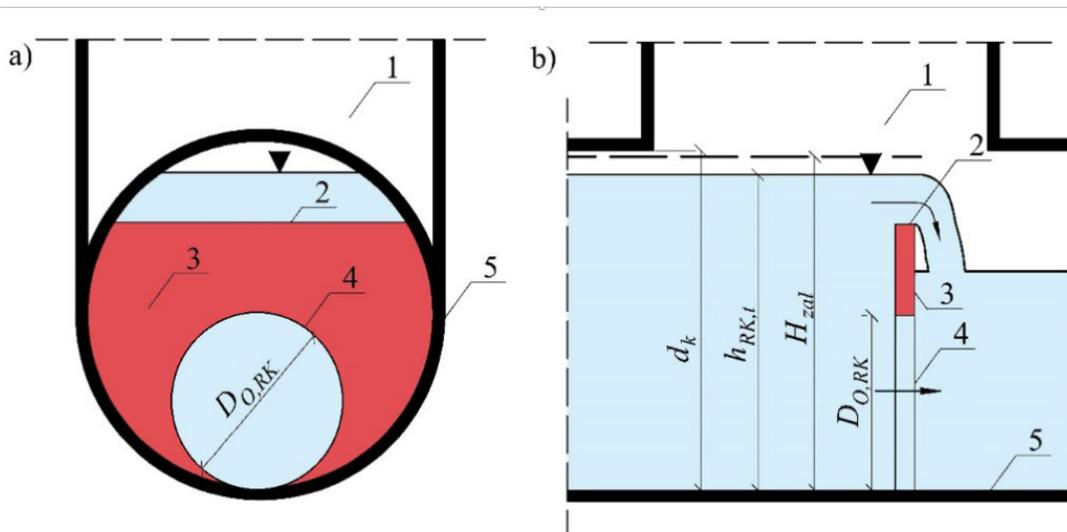
**Figure 4:** Scheme of the damming partition installed in a sewage manhole (a) cross section; (b) longitudinal section; 1 - sewer manhole, 2 - overflow edge, 3 - piling partition, 4 - flow opening, 5 - canal,  $D_{0,RK}$  - diameter of the flow opening,  $d_k$  - diameter of canal,  $h_{RK,t}$  - rainwater height in the canal during the time  $t$ ,  $H_{zdl}$  - maximum acceptable height of rainwater before the damming partition [9].
