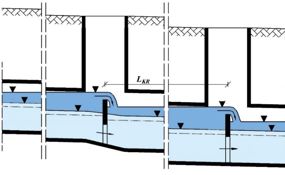
**Figure 5:** Scheme of the retention sewage canal with damming partitions that create stormwater canal retention spaces (the light blue - average distribution of the liquid stream mirror in the conduits of a traditional rainwater systems; the blue - liquid stream distribution and retention capacity of the rainwater sewage system after equipping it with damming partition),  $L_{KR}$  - distance between adjacent damming partitions [7].
