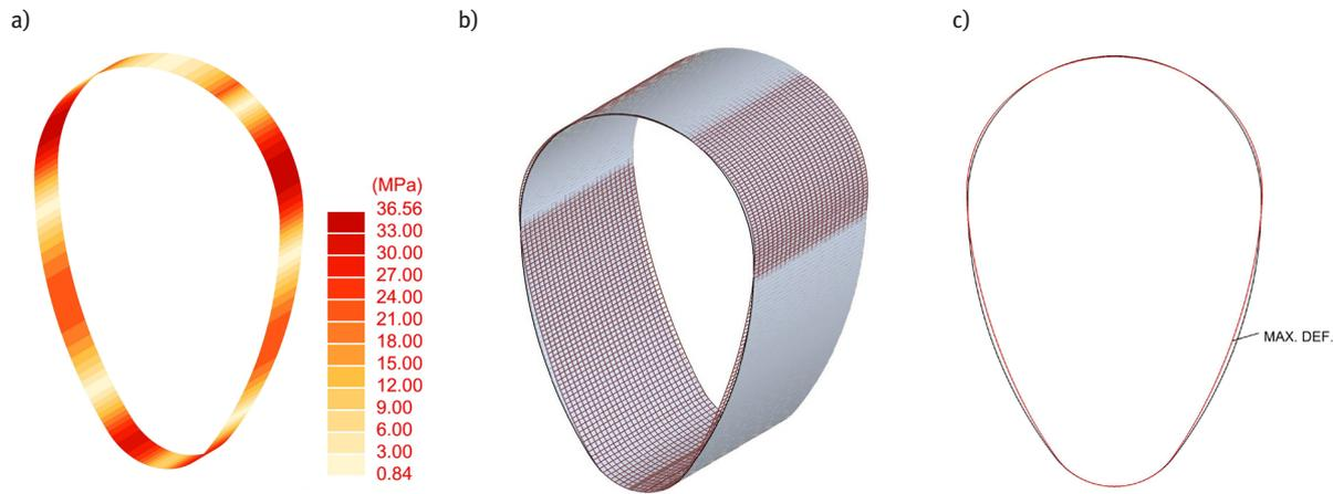
**Figure 4:** Stress distribution and deformations of the panel when the heat of hydration is equal to 25°C: (a) stress distribution, (b) 3D view of panel deformation, (c) 2D view of panel deformation with an indication of the location where the maximum value occurred.
