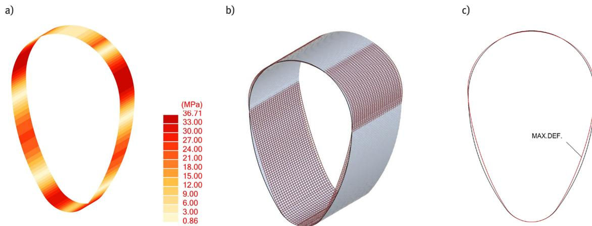
**Figure 5:** Stress distribution and deformations of the panel when the heat of hydration is equal to 40°C: (a) stress distribution, (b) 3D view of panel deformation, (c) 2D view of panel deformation with an indication of the location where the maximum value occurred.
