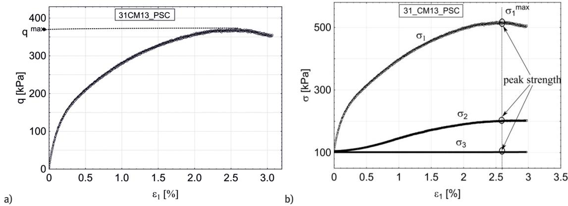
Figure 2: The principal stress and axial strain curves for the selected test in plane strain conditions: a)  $q(\varepsilon_1)$  and b)  $\sigma_1(\varepsilon_1)$ ,  $\sigma_2(\varepsilon_1)$  and  $\sigma_3(\varepsilon_1)$ .
