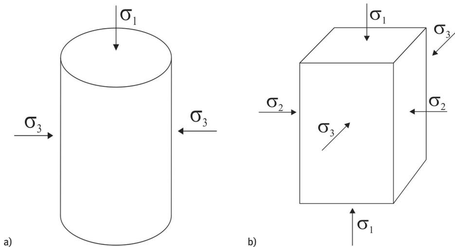
**Figure 1:** Two-dimensional and three-dimensional soil stress states: a) cylindrical sample in axisymmetric stress conditions,  $\sigma_2 = \sigma_3$  and b) rectangular sample in true triaxial conditions,  $\sigma_1 \neq \sigma_2 \neq \sigma_3$ .
