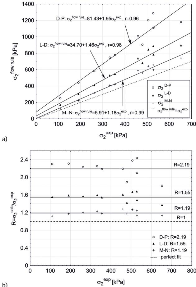
**Figure 14:** The intermediate stress  $\sigma_2$ , obtained for Drucker–Prager (D-P), Matsuoka–Nakai (M-N) and Lade–Duncan (L-D) failure criteria, assuming plane strain condition and the associated flow rule, as function of the measured  $\sigma_2$  (Table 3): (a)  $\sigma_2^{\text{calc}}(\sigma_2^{\text{exp}})$  and (b)  $R(\sigma_2^{\text{exp}})$ , where  $R = \sigma_2^{\text{calc}} / \sigma_2^{\text{exp}}$ .
