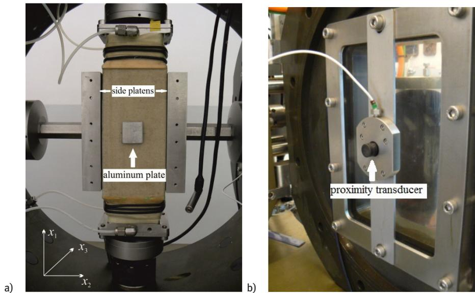
**Figure 7:** a) The GDS EMTTA chamber with a sample prepared for the test. The role of the side plates is to prevent soil deformations in the  $x_2$  direction, b) proximity transducer on the doors of the measurement cell (test chamber).
