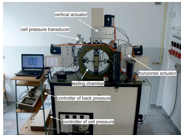
Figure 6: Components of EMTTA, used in the study.
