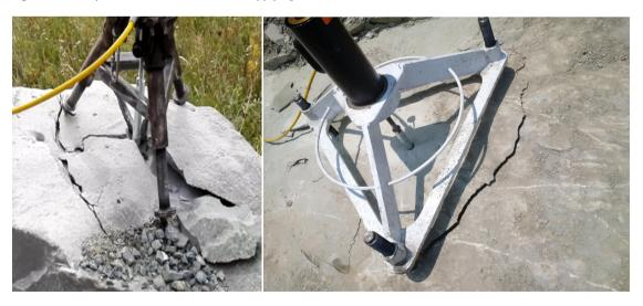
Figure 13: Pull-out test performed on actual rock (Jonak et al., 2019).
