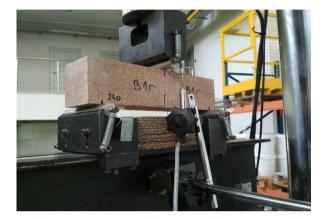
Figure 7: Three point bending test for notched beams.
