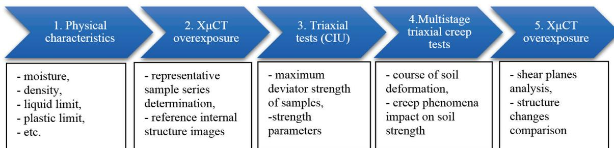
Fig. 4. Workflow of the creep deformation course study
