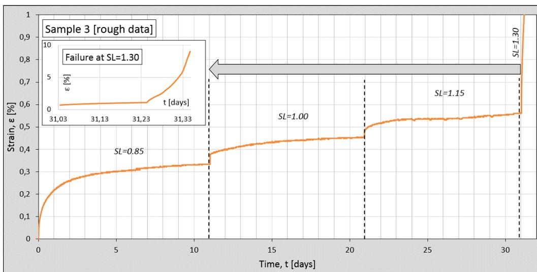
Fig. 11. The result of the multistage triaxial creep test of sample 3: A – rough data; B – data after processing
