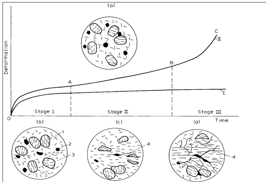
Fig. 13. Schematic representation of changes in microstructure of soil due to creep: (a) initial structure; (b) structure at stage I; (c) structure at stage II; (d) structure at stage III of creep; 1 – micro-aggregates of clay particles; 2 – cavities and voids; 3 – cementing clay; 4 – micro- and macro-cracks [33]
