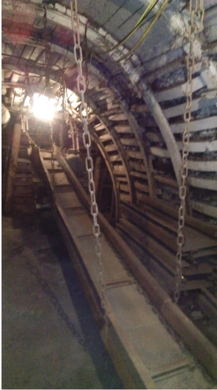
Fig. 1. The scraper conveyor in one of Polish mines (courtesy of A. Katunin)
