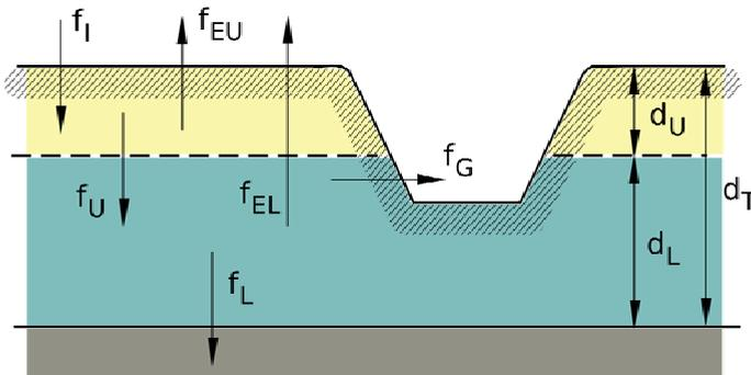
Fig. 6. Groundwater model in the SWMM program
