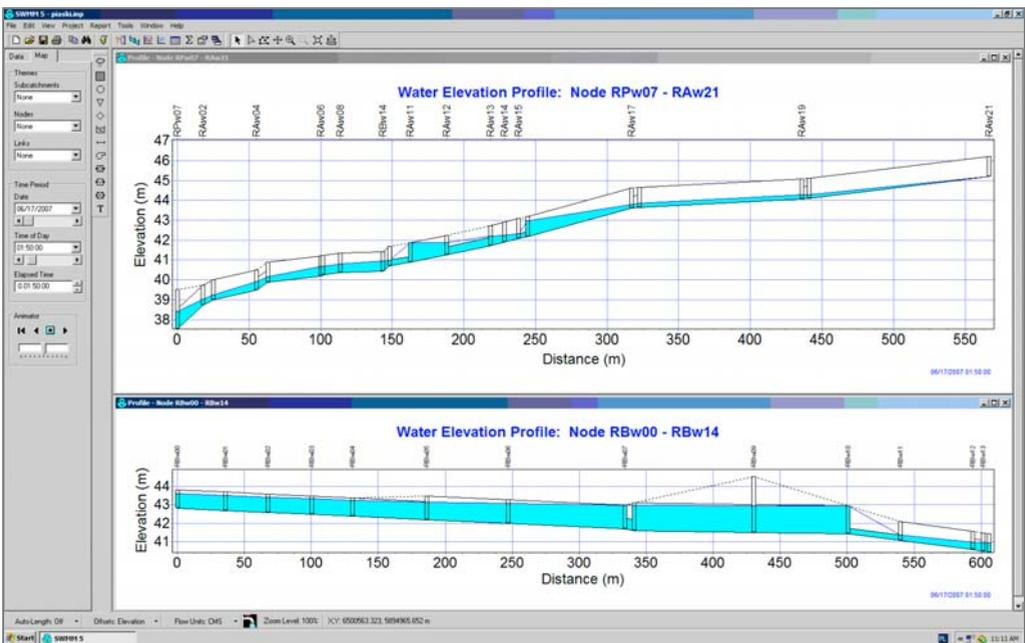
Fig. 13. Simulation results of the outflow from Piaski – Dolny Taras catchment. The profiles of RA and RB ditches. Water levels after 1 hour 50 min from the start of the simulation.
