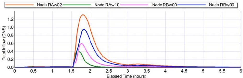
Fig. 15. Simulation results of the outflow from Piaski – Dolny Taras catchment.
