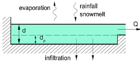
Fig. 5. Surface runoff model in SWMM program
