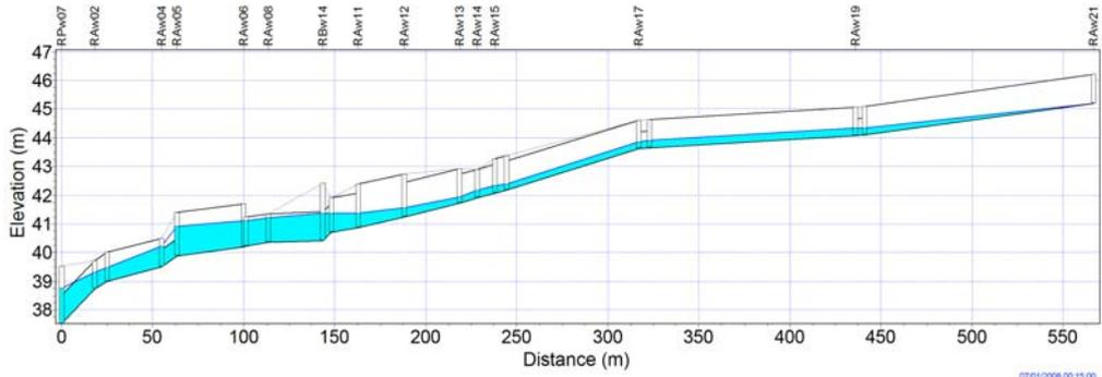
Fig. 11. Simulation results of the outflow from Piaski – Dolny Taras catchment. The profile of water levels in RA ditch after 15 minutes from the start of the rainfall. Rainfall 77.4 mm/h, lasting 10 min;  $p = 10\%$
