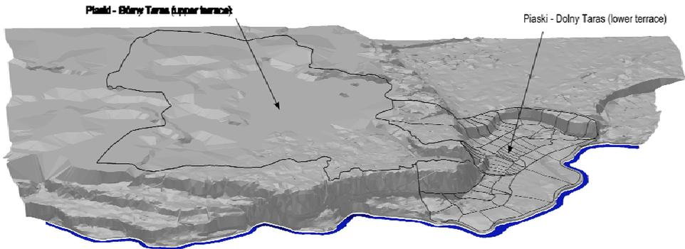
Fig. 2. The surface of the catchment axonometry; the vertical scale is 5 times the horizontal
