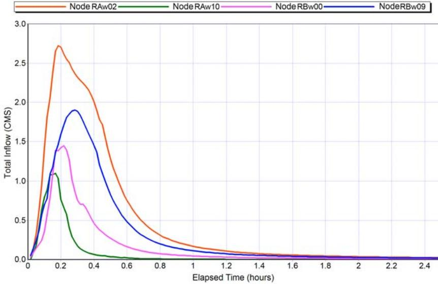
Fig. 9. Simulation results of the outflow from Piaski – Dolny Taras catchment. Discharges in the junctions. Rainfall 77.4 mm/h, lasting 10 min;  $p = 10\%$
