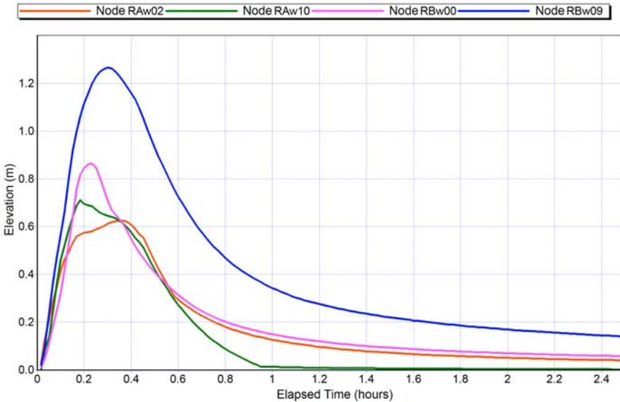
Fig. 10. Simulation results of the outflow from Piaski – Dolny Taras catchment. Water levels in the junctions. Rainfall 77.4 mm/h, lasting 10 min;  $p = 10\%$
