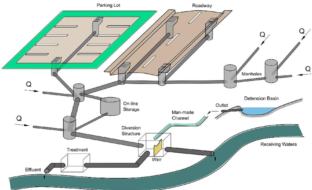
Fig. 3. Outline of the model of a drainage system in SWMM program
