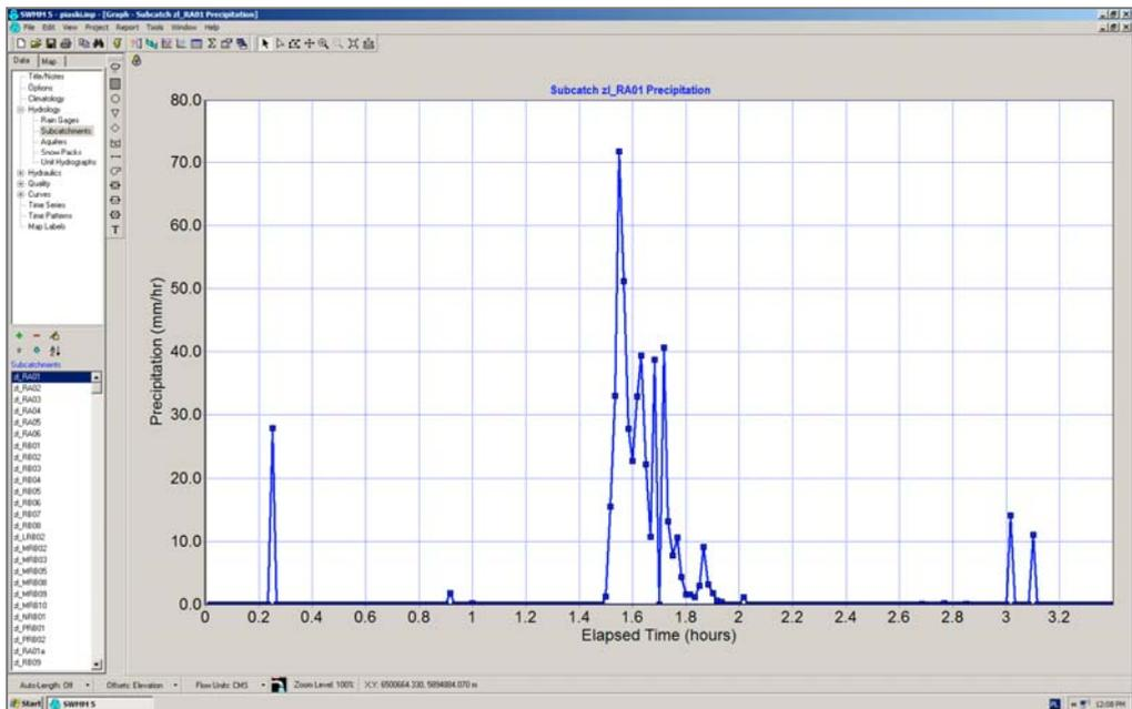
Fig. 12. Rainfall hyetograph based on the rainfall registered on 17 June 2007 at Climatological Station in Chrzastowo
