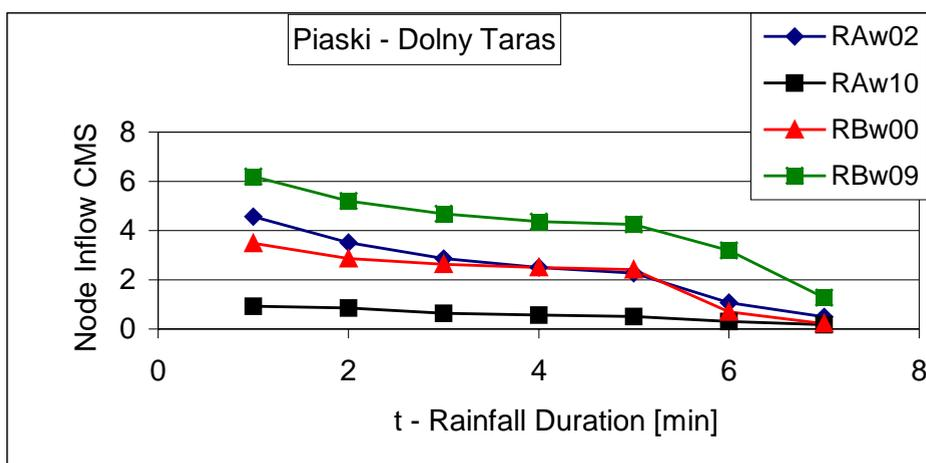
Fig. 8. Results of the flow simulation depending on the duration of the rainfall ( $t < 10$  min), at selected points of RA and RB ditches. Rainfall intensity calculated for  $p = 10\%$
