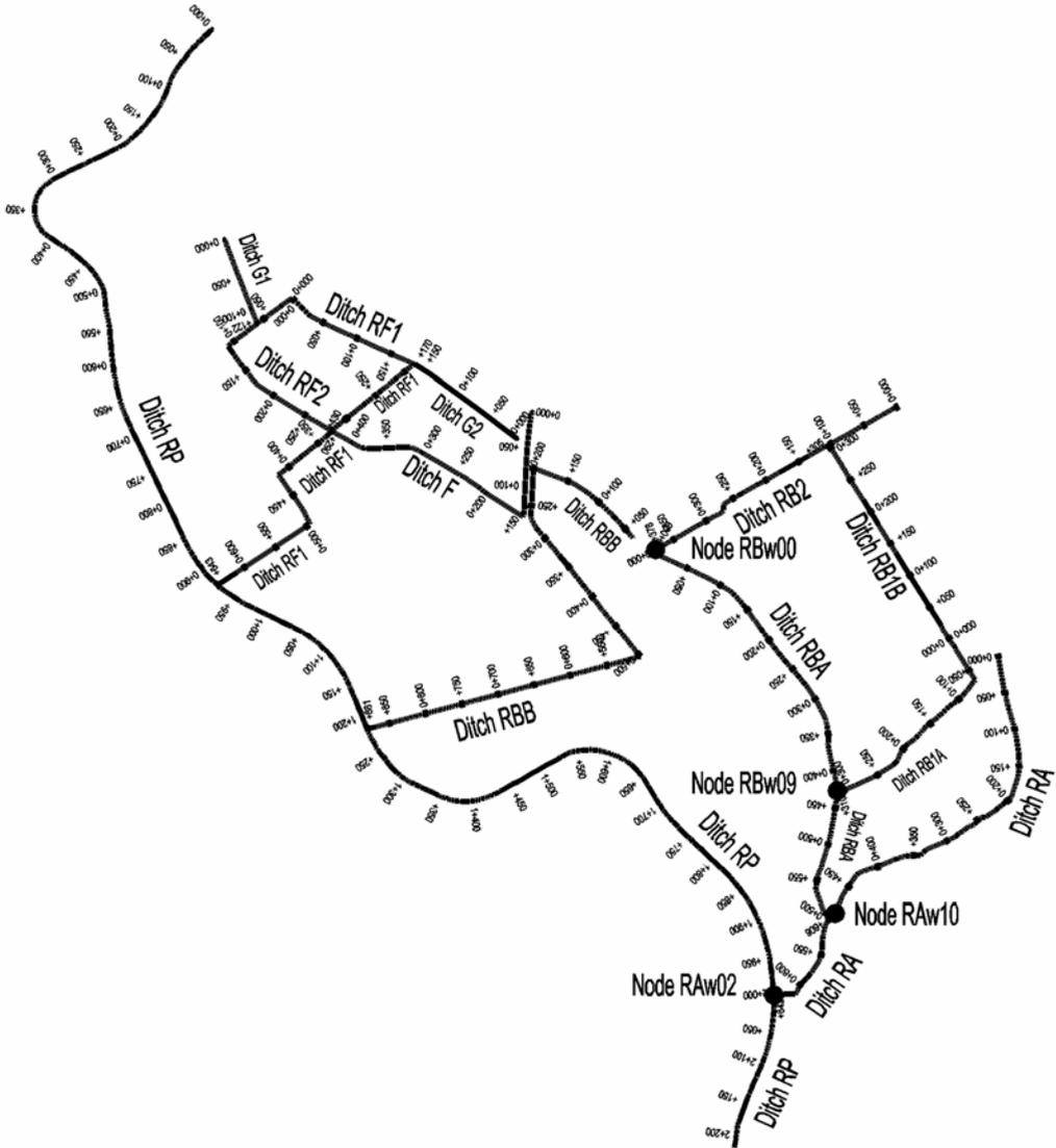
Fig. 7. The ideogram of the main conduits of Piaski – Dolny Taras estate; the names of ditches and junctions
