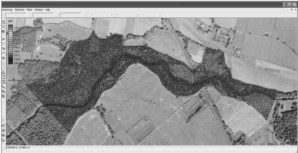
Fig. 2. 2D finite element meshes generated on the basis of DTM
