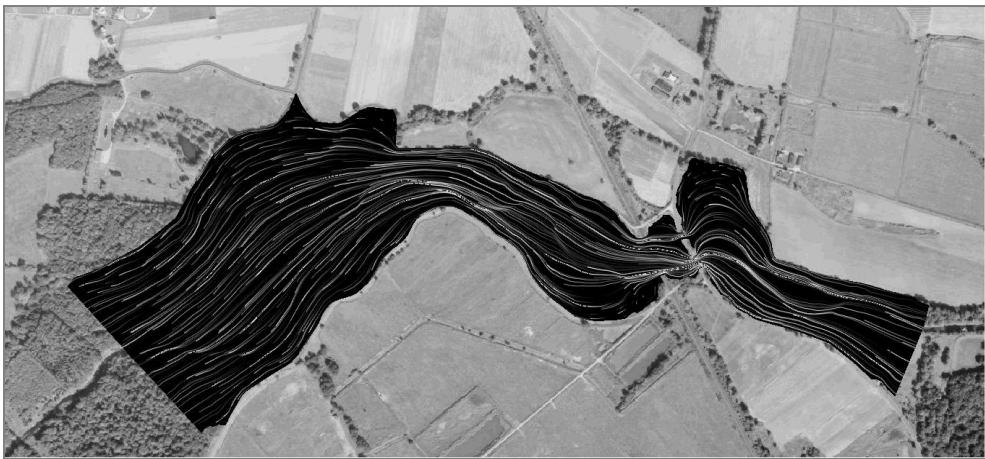
Fig. 3. Flow Trace at the modelled discharge  $Q = 130 \text{ m}^3/\text{s}$
