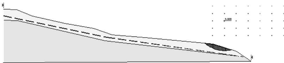
Fig. 13. Local failure circle at the bottom of slope and for homogeneous suction  $s = 40$  kPa
