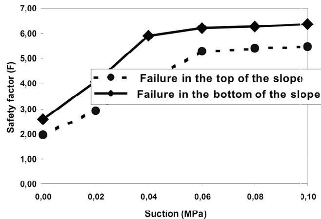
Fig. 11. Predicted safety factor versus suction obtained for the circle failure at the top and the bottom of the slope
