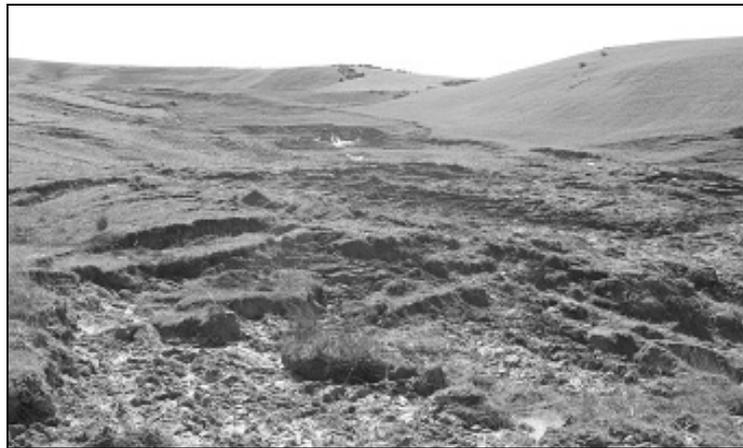
Fig. 1. Slope profile and collapse of the marly clay after the wet season (at a saturation state)
