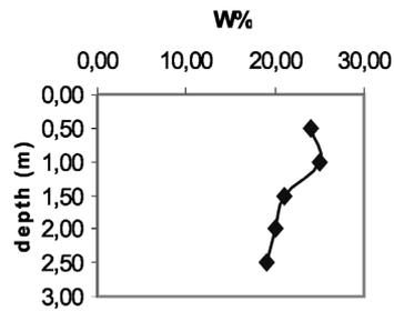
Fig. 4. Water content – depth evolution (Dec. 2006)
