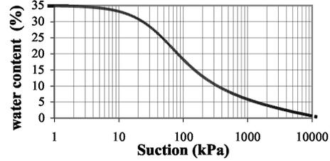
Fig. 8. Soil-water characteristic curve
