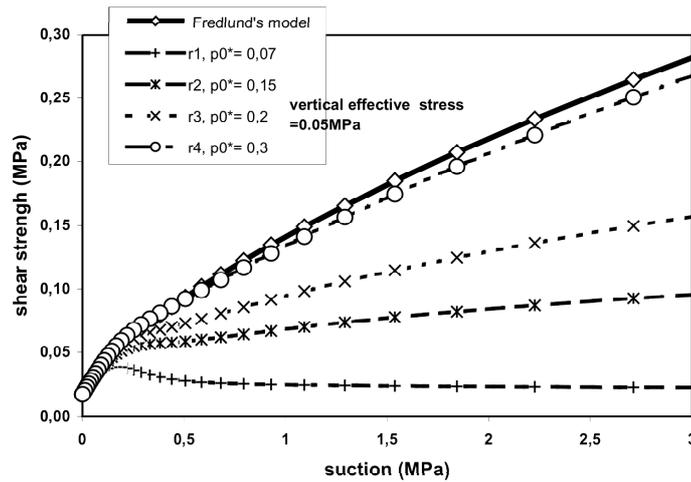
Fig. 10. Shear strength versus suction for different initial saturated preconsolidation stresses
