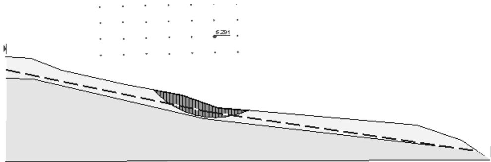
Fig. 12. Local failure circle at the top of slope and for a homogeneous suction  $s = 60$  kPa
