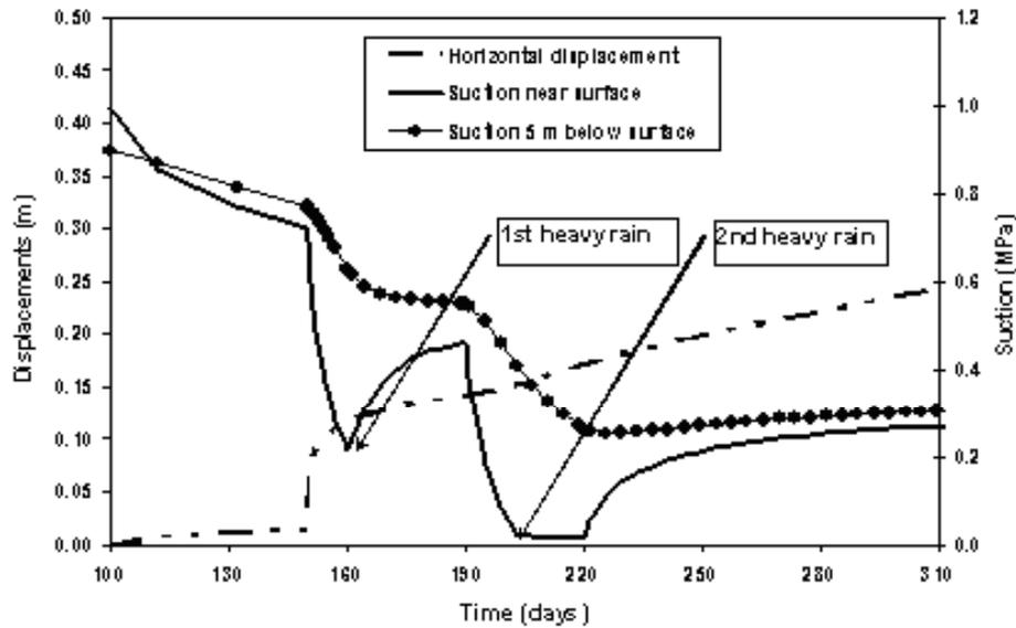
Fig. 17. Horizontal displacement and suction evolutions with time
