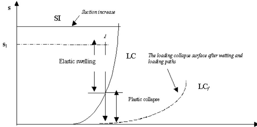
Fig. 9. The principles of the BBM model to include the collapse effect: loading-collapse (LC) and suction increase (SI) yield curves (ALONSO et al. [2])
