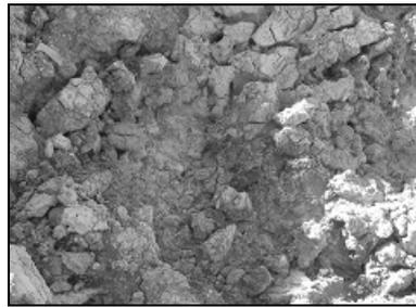
Fig. 6. Behaviour of soil collapse after wetting
