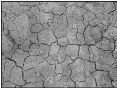
Fig. 5. Pattern cracks after drying
