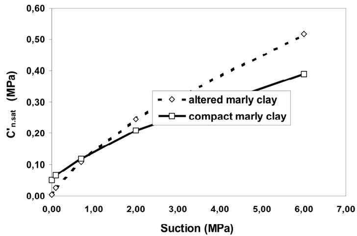
Fig. 14. The effective cohesion for the altered and compact clays
