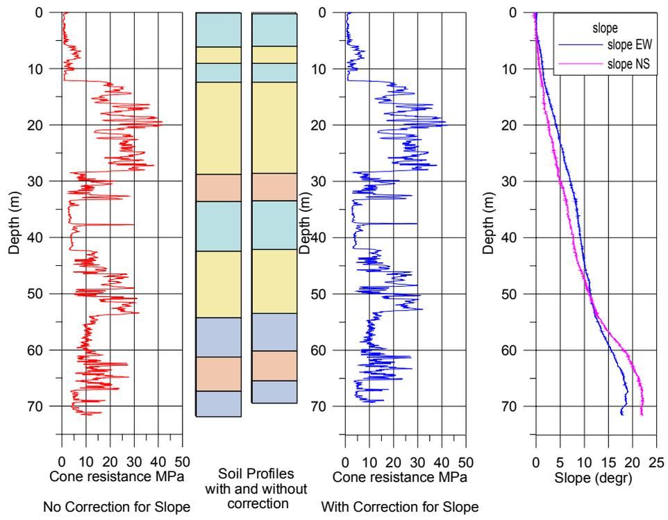
Fig. 7a. Effect of correcting penetration depth for inclination, deep profile
