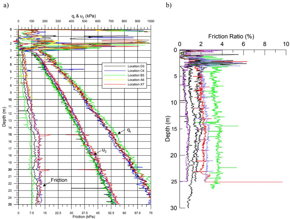
Fig. 6. Typical results showing repeatability for one cone (a),
