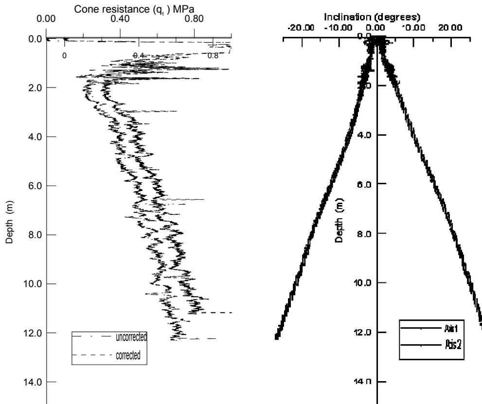
Fig. 8. Effect of correcting penetration depth for inclination, shallow depths coiled system (note axis shift in  $q_c$  to separate plots)
