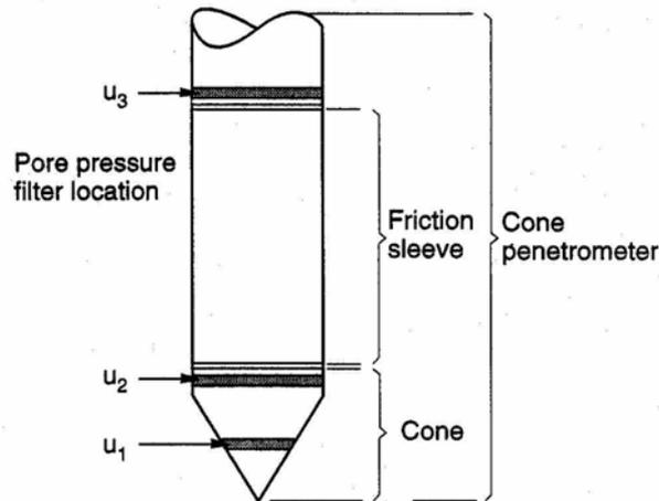
Fig. 1. Standard cone penetrometer with pore pressure measurement (CPTU)
