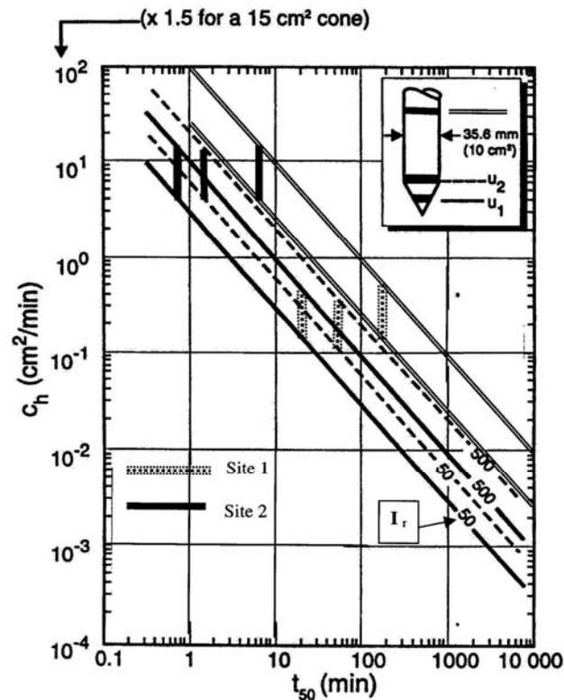
Fig. 19. Simplified plot for determining  $c_h$  from piezocone dissipation
