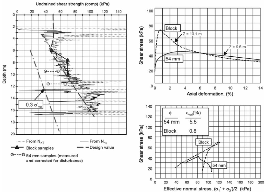
Fig. 16. Above: Undrained shear strength derived from cone penetration tests and compared with laboratory tests results on 54-mm and 250-mm block samples. Nykirke railway link (JENSEN [15])
