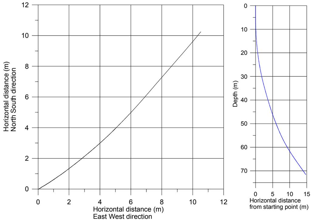
Fig. 7b. Effect of correcting penetration depth for inclination, deep profile
