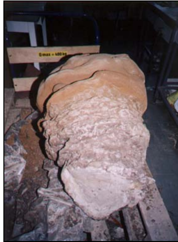
Photo 1. Jet-grouting pile after excavation and cleaning at the laboratory
